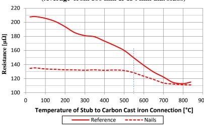
Laboratory test results of electrical resistance through full height anodes with 155.5 mm stub hole diameter. The plots include the average of 134 & 100 mm diameter stubs to reflect a normal stub population.
