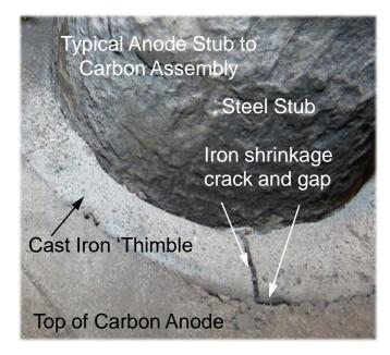
**Anode Nails**: Custom alloy hardened nails inserted into the stubhole walls, prior to anode assembly. The nails bridge the air gap to reduce electrical contact resistance. The nails are recycled by remelting with the cast iron thimble. Nails may be installed manually or robotically.
